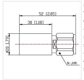
RF Solution offer a wide selection of Coaxial Fixed Termination (Dummy Load) for global customers. CT-05W-RA2030-NJ-6G is a Coaxial Fixed Termination (Dummy Load) in Frequency Range of DC~6.0 GHz. It is made of high quality materials under a high standard, the Connector Type of this product is N-M (J), VSWR Max is 1.25 and Impedance is 50  $\Omega$ . The component has a good working performance and stability, it is ideal for handling a Power of 5 W.
