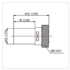
RF Solution offer a wide selection of Coaxial Fixed Termination (Dummy Load) for global customers. CT-05W-RA2030-DINK-3G is Coaxial Termination (Dummy Load) in Frequency Range of DC~3.0 GHz. It is made of high quality materials under a high standard, the Connector Type of this product is DIN-F (K), VSWR Max is 1.20 and Impedance is 50  $\Omega$ . The component has a good working performance and stability, it is ideal for handling a Power of 5 W.
