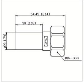
RF Solution offer a wide selection of Coaxial Fixed Termination (Dummy Load) for global customers. CT-05W-RA2030-DINJ-6G is a Coaxial Fixed Termination (Dummy Load) in Frequency Range of DC $\sim$ 6.0 GHz. It is made of high quality materials under a high standard, the Connector Type of this product is DIN-M (J), VSWR Max is 1.30 and Impedance is 50  $\Omega$ . The component has a good working performance and stability, it is ideal for handling a Power of 5 W.
