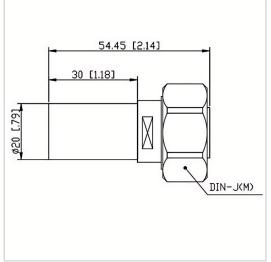
RF Solution offer a wide selection of Coaxial Fixed Termination (Dummy Load) for global customers. CT-05W-RA2030-DINJ-3G is a Coaxial Fixed Termination (Dummy Load) in Frequency Range of DC $\sim$ 3.0 GHz. It is made of high quality materials under a high standard, the Connector Type of this product is 4.3-10-F (K), VSWR Max is 1.20 and Impedance is 50  $\Omega$ . The component has a good working performance and stability, it is ideal for handling a Power of 5 W.
