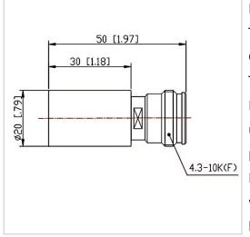
RF Solution offer a wide selection of Coaxial Fixed Termination (Dummy Load) for global customers. CT-05W-RA2030-4310K-4G is a Coaxial Fixed Termination (Dummy Load) in Frequency Range of DC~4.0 GHz. It is made of high quality materials under a high standard, the Connector Type of this product is 4.3-10-F (K), VSWR Max is 1.25 and Impedance is 50  $\Omega$ . The component has a good working performance and stability, it is ideal for handling a Power of 5 W.
