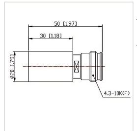
RF Solution offer a wide selection of Coaxial Fixed Termination (Dummy Load) for global customers. CT-05W-RA2030-4310K-3G is a Coaxial Fixed Termination (Dummy Load) in Frequency Range of DC~3.0 GHz. It is made of high quality materials under a high standard, the Connector Type of this product is 4.3-10-F (K), VSWR Max is 1.20 and Impedance is 50  $\Omega$ . The component has a good working performance and stability, it is ideal for handling a Power of 5 W.
