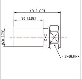
RF Solution offer a wide selection of Coaxial Fixed Termination (Dummy Load) for global customers. CT-05W-RA2030-4310J-6G is а Coaxial Termination (Dummy Load) in Frequency Range of DC~6.0 GHz. It is made of high quality materials under a high standard, the Connector Type of this product is 4.3-10-M (J), VSWR Max is 1.30 and Impedance is 50  $\Omega$ . The component has a good working performance and stability, it is ideal for handling a Power of 5 W.
