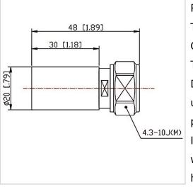
RF Solution offer a wide selection of Coaxial Fixed Termination (Dummy Load) for global customers. CT-05W-RA2030-4310J-4G is a Coaxial Fixed Termination (Dummy Load) in Frequency Range of DC~4.0 GHz. It is made of high quality materials under a high standard, the Connector Type of this product is 4.3-10-M (J), VSWR Max is 1.25 and Impedance is 50  $\Omega$ . The component has a good working performance and stability, it is ideal for handling a Power of 5 W.
