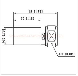
RF Solution offer a wide selection of Coaxial Fixed Termination (Dummy Load) for global customers. CT-05W-RA2030-4310J-3G is a Coaxial Fixed Termination (Dummy Load) in Frequency Range of DC $\sim$ 3.0 GHz. It is made of high quality materials under a high standard, the Connector Type of this product is 4.3-10-M (J), VSWR Max is 1.20 and Impedance is 50  $\Omega$ . The component has a good working performance and stability, it is ideal for handling a Power of 5 W.
