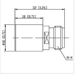
RF Solution offer a wide selection of Coaxial Fixed Termination (Dummy Load) for global customers. CT-05W-RA1818-NK-18G is Coaxial Fixed Termination (Dummy Load) in Frequency Range of DC~18.0 GHz. It is made of high quality materials under a high standard, the Connector Type of this product is N-F (K), VSWR Max is 1.30 and Impedance is 50  $\Omega$ . The component has a good working performance and stability, it is ideal for handling a Power of 5 W.
