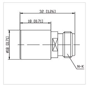
RF Solution offer a wide selection of Coaxial Fixed Termination (Dummy Load) for global customers. CT-05W-RA1818-NK-12.4G is a Coaxial Fixed Termination (Dummy Load) in Frequency Range of DC~12.4 GHz. It is made of high quality materials under a high standard, the Connector Type of this product is N-F (K), VSWR Max is 1.25 and Impedance is 50  $\Omega$ . The component has a good working performance and stability, it is ideal for handling a Power of 5 W.
