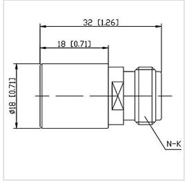
RF Solution offer a wide selection of Coaxial Fixed Termination (Dummy Load) for global customers. CT-05W-RA1818-NK-10G is Coaxial Fixed а Termination (Dummy Load) in Frequency Range of DC~10.0 GHz. It is made of high quality materials under a high standard, the Connector Type of this product is N-F (K), VSWR Max is 1.25 and Impedance is 50  $\Omega$ . The component has a good working performance and stability, it is ideal for handling a Power of 5 W.
