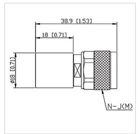
RF Solution offer a wide selection of Coaxial Fixed Termination (Dummy Load) for global customers. CT-05W-RA1818-NJ-8G is a Coaxial Fixed Termination (Dummy Load) in Frequency Range of DC~8.0 GHz. It is made of high quality materials under a high standard, the Connector Type of this product is N-M (J), VSWR Max is 1.20 and Impedance is 50  $\Omega$ . The component has a good working performance and stability, it is ideal for handling a Power of 5 W.
