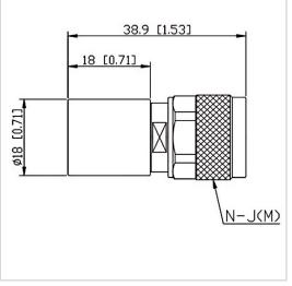
RF Solution offer a wide selection of Coaxial Fixed Termination (Dummy Load) for global customers. CT-05W-RA1818-NJ-18G is a Coaxial Fixed Termination (Dummy Load) in Frequency Range of DC~18.0 GHz. It is made of high quality materials under a high standard, the Connector Type of this product is N-M (J), VSWR Max is 1.30 and Impedance is 50  $\Omega$ . The component has a good working performance and stability, it is ideal for handling a Power of 5 W.
