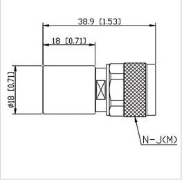
RF Solution offer a wide selection of Coaxial Fixed Termination (Dummy Load) for global customers. CT-05W-RA1818-NJ-12.4G is a Coaxial Fixed Termination (Dummy Load) in Frequency Range of DC~12.4 GHz. It is made of high quality materials under a high standard, the Connector Type of this product is N-M (J), VSWR Max is 1.25 and Impedance is 50  $\Omega$ . The component has a good working performance and stability, it is ideal for handling a Power of 5 W.
