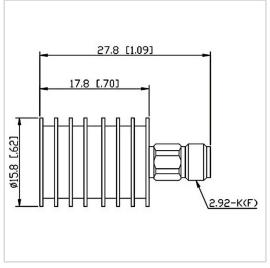
RF Solution offer a wide selection of Coaxial Fixed Termination (Dummy Load) for global customers. CT-05W-RA1618-2.92K-40G is a Coaxial Fixed Termination (Dummy Load) in Frequency Range of DC~40.0 GHz. It is made of high quality materials under a high standard, the Connector Type of this product is 2.92-F (K), VSWR Max is 1.25 and Impedance is 50  $\Omega$ . The component has a good working performance and stability, it is ideal for handling a Power of 5 W.
