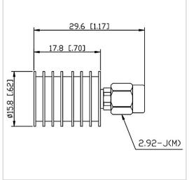
RF Solution offer a wide selection of Coaxial Fixed Termination (Dummy Load) for global customers. CT-05W-RA1618-2.92J-40G is a Coaxial Fixed Termination (Dummy Load) in Frequency Range of DC~40.0 GHz. It is made of high quality materials under a high standard, the Connector Type of this product is 2.92-M (J), VSWR Max is 1.25 and Impedance is 50  $\Omega$ . The component has a good working performance and stability, it is ideal for handling a Power of 5 W.
