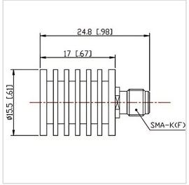
RF Solution offer a wide selection of Coaxial Fixed Termination (Dummy Load) for global customers. CT-05W-RA1517-SK-8G is a Coaxial Fixed Termination (Dummy Load) in Frequency Range of DC~8.0 GHz. It is made of high quality materials under a high standard, the Connector Type of this product is SMA-F (K), VSWR Max is 1.25 and Impedance is 50  $\Omega$ . The component has a good working performance and stability, it is ideal for handling a Power of 5 W.
