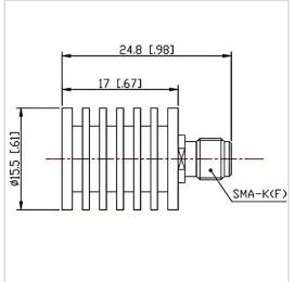
RF Solution offer a wide selection of Coaxial Fixed Termination (Dummy Load) for global customers. CT-05W-RA1517-SK-6G is a Coaxial Fixed Termination (Dummy Load) in Frequency Range of DC $\sim$ 6.0 GHz. It is made of high quality materials under a high standard, the Connector Type of this product is SMA-F (K), VSWR Max is 1.25 and Impedance is 50  $\Omega$ . The component has a good working performance and stability, it is ideal for handling a Power of 5 W.
