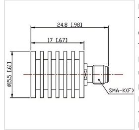
RF Solution offer a wide selection of Coaxial Fixed Termination (Dummy Load) for global customers. CT-05W-RA1517-SK-4G is a Coaxial Fixed Termination (Dummy Load) in Frequency Range of DC~4.0 GHz. It is made of high quality materials under a high standard, the Connector Type of this product is SMA-F (K), VSWR Max is 1.25 and Impedance is 50  $\Omega$ . The component has a good working performance and stability, it is ideal for handling a Power of 5 W.
