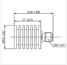
RF Solution offer a wide selection of Coaxial Fixed Termination (Dummy Load) for global customers. CT-05W-RA1517-SK-3G is Coaxial Fixed а Termination (Dummy Load) in Frequency Range of DC~3.0 GHz. It is made of high quality materials under a high standard, the Connector Type of this product is SMA-F (K), VSWR Max is 1.20 and Impedance is 50  $\Omega$ . The component has a good working performance and stability, it is ideal for handling a Power of 5 W.
