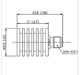
RF Solution offer a wide selection of Coaxial Fixed Termination (Dummy Load) for global customers. CT-05W-RA1517-SK-18G is a Coaxial Fixed Termination (Dummy Load) in Frequency Range of DC~18.0 GHz. It is made of high quality materials under a high standard, the Connector Type of this product is SMA-F (K), VSWR Max is 1.30 and Impedance is 50  $\Omega$ . The component has a good working performance and stability, it is ideal for handling a Power of 5 W.
