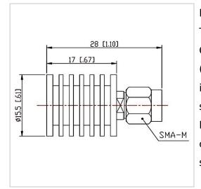
RF Solution offer a wide selection of Coaxial Fixed Termination (Dummy Load) for global customers. CT-05W-RA1517-SJ-8G is a Coaxial Fixed Termination (Dummy Load) in Frequency Range of DC~8.0 GHz. It is made of high quality materials under a high standard, the Connector Type of this product is SMA-M (J), VSWR Max is 1.20 and Impedance is 50  $\Omega$ . The component has a good working performance and stability, it is ideal for handling a Power of 5 W.
