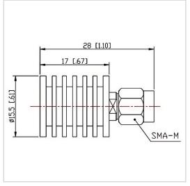
RF Solution offer a wide selection of Coaxial Fixed Termination (Dummy Load) for global customers. CT-05W-RA1517-SJ-6G is a Coaxial Fixed Termination (Dummy Load) in Frequency Range of DC~6.0 GHz. It is made of high quality materials under a high standard, the Connector Type of this product is SMA-M (J), VSWR Max is 1.25 and Impedance is 50  $\Omega$ . The component has a good working performance and stability, it is ideal for handling a Power of 5 W.
