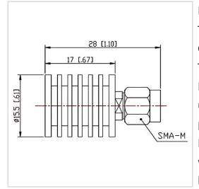
RF Solution offer a wide selection of Coaxial Fixed Termination (Dummy Load) for global customers. CT-05W-RA1517-SJ-18G is a Coaxial Fixed Termination (Dummy Load) in Frequency Range of DC~18.0 GHz. It is made of high quality materials under a high standard, the Connector Type of this product is SMA-M (J), VSWR Max is 1.30 and Impedance is 50  $\Omega$ . The component has a good working performance and stability, it is ideal for handling a Power of 5 W.
