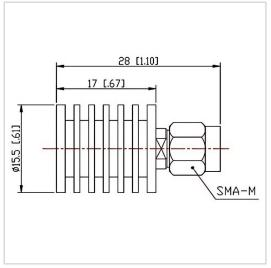
RF Solution offer a wide selection of Coaxial Fixed Termination (Dummy Load) for global customers. CT-05W-RA1517-SJ-12.4G is a Coaxial Fixed Termination (Dummy Load) in Frequency Range of DC~12.4 GHz. It is made of high quality materials under a high standard, the Connector Type of this product is SMA-M (J), VSWR Max is 1.25 and Impedance is 50  $\Omega$ . The component has a good working performance and stability, it is ideal for handling a Power of 5 W.
