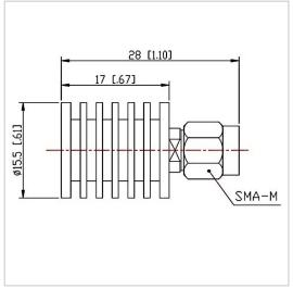
RF Solution offer a wide selection of Coaxial Fixed Termination (Dummy Load) for global customers. CT-05W-RA1517-SJ-10G is a Coaxial Fixed Termination (Dummy Load) in Frequency Range of DC~10.0 GHz. It is made of high quality materials under a high standard, the Connector Type of this product is SMA-M (J), VSWR Max is 1.25 and Impedance is 50  $\Omega$ . The component has a good working performance and stability, it is ideal for handling a Power of 5 W.
