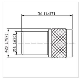
RF Solution offer a wide selection of Coaxial Fixed Termination (Dummy Load) for global customers. CT-02W-RF2036-NJ-4G is a Coaxial Fixed Termination (Dummy Load) in Frequency Range of DC $\sim$ 4.0 GHz. It is made of high quality materials under a high standard, the Connector Type of this product is N-M (J), VSWR Max is 1.20 and Impedance is 50  $\Omega$ . The component has a good working performance and stability, it is ideal for handling a Power of 2 W.
