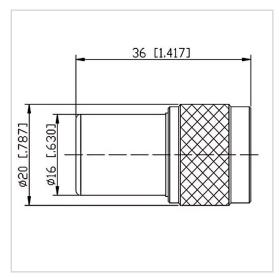
RF Solution offer a wide selection of Coaxial Fixed Termination (Dummy Load) for global customers. CT-02W-RF2036-NJ-3G is a Coaxial Fixed Termination (Dummy Load) in Frequency Range of DC $\sim$ 3.0 GHz. It is made of high quality materials under a high standard, the Connector Type of this product is N-M (J), VSWR Max is 1.20 and Impedance is 50  $\Omega$ . The component has a good working performance and stability, it is ideal for handling a Power of 2 W.
