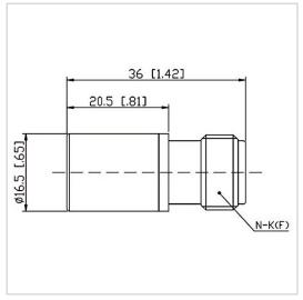
RF Solution offer a wide selection of Coaxial Fixed Termination (Dummy Load) for global customers. CT-02W-RF1620-NK-4G is Coaxial Fixed а Termination (Dummy Load) in Frequency Range of DC~4.0 GHz. It is made of high quality materials under a high standard, the Connector Type of this product is N-F (K), VSWR Max is 1.25 and Impedance is 50  $\Omega$ . The component has a good working performance and stability, it is ideal for handling a Power of 2 W.
