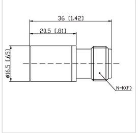
RF Solution offer a wide selection of Coaxial Fixed Termination (Dummy Load) for global customers. CT-02W-RF1620-NK-3G is a Coaxial Fixed Termination (Dummy Load) in Frequency Range of DC $\sim$ 3.0 GHz. It is made of high quality materials under a high standard, the Connector Type of this product is N-F (K), VSWR Max is 1.20 and Impedance is 50  $\Omega$ . The component has a good working performance and stability, it is ideal for handling a Power of 2 W.
