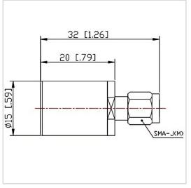
RF Solution offer a wide selection of Coaxial Fixed Termination (Dummy Load) for global customers. CT-02W-RF1520-SJ-4G is a Coaxial Fixed Termination (Dummy Load) in Frequency Range of DC~4.0 GHz. It is made of high quality materials under a high standard, the Connector Type of this product is SMA-M (J), VSWR Max is 1.20 and Impedance is 50  $\Omega$ . The component has a good working performance and stability, it is ideal for handling a Power of 2 W.
