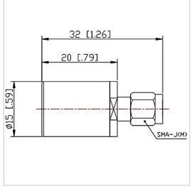
RF Solution offer a wide selection of Coaxial Fixed Termination (Dummy Load) for global customers. CT-02W-RF1520-SJ-3G is a Coaxial Fixed Termination (Dummy Load) in Frequency Range of DC~3.0 GHz. It is made of high quality materials under a high standard, the Connector Type of this product is SMA-M (J), VSWR Max is 1.20 and Impedance is 50  $\Omega$ . The component has a good working performance and stability, it is ideal for handling a Power of 2 W.
