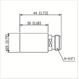
RF Solution offer a wide selection of Coaxial Fixed Termination (Dummy Load) for global customers. CT-02W-RA2030-NK-6G is Coaxial Fixed а Termination (Dummy Load) in Frequency Range of DC~6.0 GHz. It is made of high quality materials under a high standard, the Connector Type of this product is N-F (K), VSWR Max is 1.25 and Impedance is 50  $\Omega$ . The component has a good working performance and stability, it is ideal for handling a Power of 2 W.
