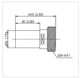
RF Solution offer a wide selection of Coaxial Fixed Termination (Dummy Load) for global customers. CT-02W-RA2030-DINK-6G is Coaxial Termination (Dummy Load) in Frequency Range of DC~6.0 GHz. It is made of high quality materials under a high standard, the Connector Type of this product is DIN-F (K), VSWR Max is 1.30 and Impedance is 50  $\Omega$ . The component has a good working performance and stability, it is ideal for handling a Power of 2 W.
