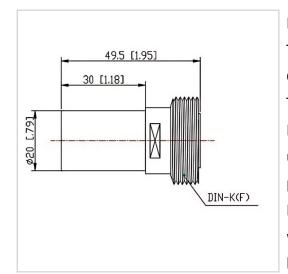
RF Solution offer a wide selection of Coaxial Fixed Termination (Dummy Load) for global customers. CT-02W-RA2030-DINK-4G is a Coaxial Fixed Termination (Dummy Load) in Frequency Range of DC~4.0 GHz. It is made of high quality materials under a high standard, the Connector Type of this product is DIN-F (K), VSWR Max is 1.25 and Impedance is 50  $\Omega$ . The component has a good working performance and stability, it is ideal for handling a Power of 2 W.
