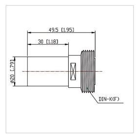
RF Solution offer a wide selection of Coaxial Fixed Termination (Dummy Load) for global customers. CT-02W-RA2030-DINK-3G is a Coaxial Fixed Termination (Dummy Load) in Frequency Range of DC $\sim$ 3.0 GHz. It is made of high quality materials under a high standard, the Connector Type of this product is DIN-F (K), VSWR Max is 1.20 and Impedance is 50  $\Omega$ . The component has a good working performance and stability, it is ideal for handling a Power of 2 W.
