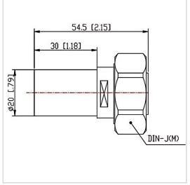
RF Solution offer a wide selection of Coaxial Fixed Termination (Dummy Load) for global customers. CT-02W-RA2030-DINJ-6G is а Coaxial Termination (Dummy Load) in Frequency Range of DC~4.0 GHz. It is made of high quality materials under a high standard, the Connector Type of this product is DIN-M (J), VSWR Max is 1.25 and Impedance is 50  $\Omega$ . The component has a good working performance and stability, it is ideal for handling a Power of 2 W.
