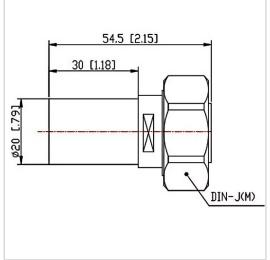
RF Solution offer a wide selection of Coaxial Fixed Termination (Dummy Load) for global customers. CT-02W-RA2030-DINJ-4G is а Coaxial Termination (Dummy Load) in Frequency Range of DC~4.0 GHz. It is made of high quality materials under a high standard, the Connector Type of this product is DIN-M (J), VSWR Max is 1.25 and Impedance is 50  $\Omega$ . The component has a good working performance and stability, it is ideal for handling a Power of 2 W.
