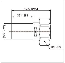
RF Solution offer a wide selection of Coaxial Fixed Termination (Dummy Load) for global customers. CT-02W-RA2030-DINJ-3G is a Coaxial Fixed Termination (Dummy Load) in Frequency Range of DC~3.0 GHz. It is made of high quality materials under a high standard, the Connector Type of this product is DIN-M (J), VSWR Max is 1.20 and Impedance is 50  $\Omega$ . The component has a good working performance and stability, it is ideal for handling a Power of 2 W.
