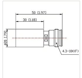
RF Solution offer a wide selection of Coaxial Fixed Termination (Dummy Load) for global customers. CT-02W-RA2030-4310K-4G is a Coaxial Fixed Termination (Dummy Load) in Frequency Range of DC~4.0 GHz. It is made of high quality materials under a high standard, the Connector Type of this product is 4.3-10-F (K), VSWR Max is 1.20 and Impedance is 50  $\Omega$ . The component has a good working performance and stability, it is ideal for handling a Power of 2 W.
