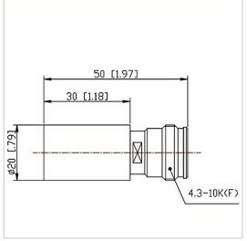
RF Solution offer a wide selection of Coaxial Fixed Termination (Dummy Load) for global customers. CT-02W-RA2030-4310K-3G is a Coaxial Fixed Termination (Dummy Load) in Frequency Range of DC $\sim$ 3.0 GHz. It is made of high quality materials under a high standard, the Connector Type of this product is 4.3-10-F (K), VSWR Max is 1.20 and Impedance is 50  $\Omega$ . The component has a good working performance and stability, it is ideal for handling a Power of 2 W.
