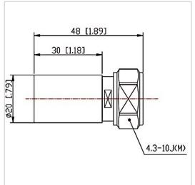
RF Solution offer a wide selection of Coaxial Fixed Termination (Dummy Load) for global customers. CT-02W-RA2030-4310J-6G is a Coaxial Fixed Termination (Dummy Load) in Frequency Range of DC~6.0 GHz. It is made of high quality materials under a high standard, the Connector Type of this product is 4.3-10-M (J), VSWR Max is 1.25 and Impedance is 50  $\Omega$ . The component has a good working performance and stability, it is ideal for handling a Power of 2 W.
