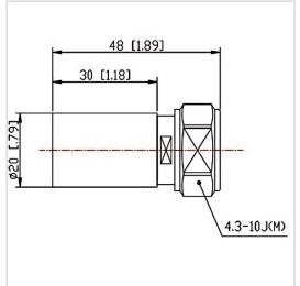
RF Solution offer a wide selection of Coaxial Fixed Termination (Dummy Load) for global customers. CT-02W-RA2030-4310J-3G is a Coaxial Fixed Termination (Dummy Load) in Frequency Range of DC~3.0 GHz. It is made of high quality materials under a high standard, the Connector Type of this product is 4.3-10-M (J), VSWR Max is 1.20 and Impedance is 50  $\Omega$ . The component has a good working performance and stability, it is ideal for handling a Power of 2 W.
