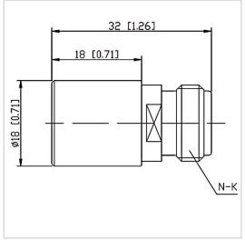
RF Solution offer a wide selection of Coaxial Fixed Termination (Dummy Load) for global customers. CT-02W-RA1818-NK-18G is Coaxial Fixed а Termination (Dummy Load) in Frequency Range of DC~18.0 GHz. It is made of high quality materials under a high standard, the Connector Type of this product is N-F (K), VSWR Max is 1.30 and Impedance is 50  $\Omega$ . The component has a good working performance and stability, it is ideal for handling a Power of 2 W.
