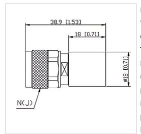
RF Solution offer a wide selection of Coaxial Fixed Termination (Dummy Load) for global customers. CT-02W-RA1818-NJ-12.4G is a Coaxial Fixed Termination (Dummy Load) in Frequency Range of DC~12.4 GHz. It is made of high quality materials under a high standard, the Connector Type of this product is N-M (J), VSWR Max is 1.25 and Impedance is 50  $\Omega$ . The component has a good working performance and stability, it is ideal for handling a Power of 2 W.
