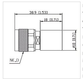
RF Solution offer a wide selection of Coaxial Fixed Termination (Dummy Load) for global customers. CT-02W-RA1818-NJ-10G is a Coaxial Fixed Termination (Dummy Load) in Frequency Range of DC~10.0 GHz. It is made of high quality materials under a high standard, the Connector Type of this product is N-M (J), VSWR Max is 1.25 and Impedance is 50  $\Omega$ . The component has a good working performance and stability, it is ideal for handling a Power of 2 W.
