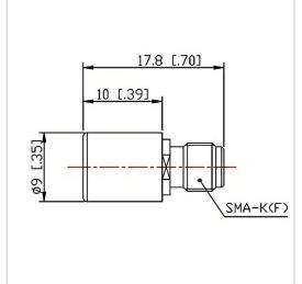
RF Solution offer a wide selection of Coaxial Fixed Termination (Dummy Load) for global customers. CT-02W-RA0910-SK-8G is a Coaxial Fixed Termination (Dummy Load) in Frequency Range of DC~8.0 GHz. It is made of high quality materials under a high standard, the Connector Type of this product is SMA-F (K), VSWR Max is 1.20 and Impedance is 50  $\Omega$ . The component has a good working performance and stability, it is ideal for handling a Power of 2 W.
