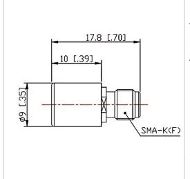
RF Solution offer a wide selection of Coaxial Fixed Termination (Dummy Load) for global customers. CT-02W-RA0910-SK-6G is a Coaxial Fixed Termination (Dummy Load) in Frequency Range of DC~6.0 GHz. It is made of high quality materials under a high standard, the Connector Type of this product is SMA-F (K), VSWR Max is 1.20 and Impedance is 50  $\Omega$ . The component has a good working performance and stability, it is ideal for handling a Power of 2 W.
