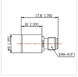
RF Solution offer a wide selection of Coaxial Fixed Termination (Dummy Load) for global customers. CT-02W-RA0910-SK-3G is a Coaxial Fixed Termination (Dummy Load) in Frequency Range of DC $\sim$ 3.0 GHz. It is made of high quality materials under a high standard, the Connector Type of this product is SMA-F (K), VSWR Max is 1.20 and Impedance is 50  $\Omega$ . The component has a good working performance and stability, it is ideal for handling a Power of 2 W.
